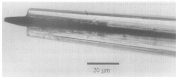
Fig. 1. A multibarreled carbon fiber microiontophoretic assembly. Four drug ejection barrels surround the carbon fiber containing barrel. The pointed tip was produced by etching with AC current in normal saline solution.
